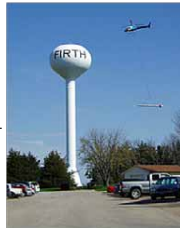
Helicopter gathering Electromagnetic data
